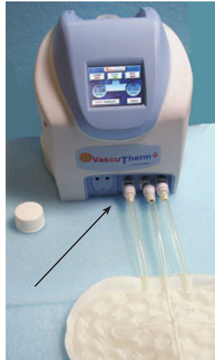
Connect therapy wrap directly to unit.
