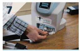
Plug the three tubes into the front of the machine. You will hear a click once all connections are secured.
